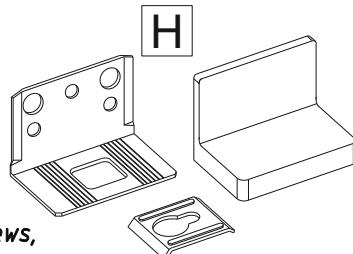
The set of accessories includes a canopy with a plug for attaching the module to the wall.
